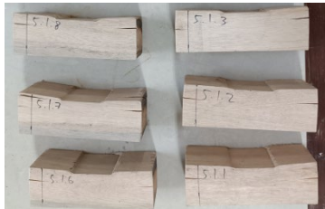
Figure 9. Results of failure mode for some 50 x 50 x 150mm specimens (compression perpendicular to the grain method of test)
