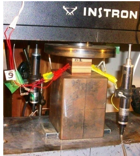
Figure 4. Setting up compression test in RL plane
