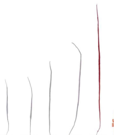
Figure 1. Morphology of wood fibers of five species from natural forest. Left to right: mentawa ( Artocarpus rigidus Blume), Cempaka ( Michelia champaca Linn), kempili ( Lithocarpus elegans (Blume) Hatus. Ex Soepadmo), menjalin ( Xanthophyllum excelsum Miq.), and sempori ( Dillenia sp.)
