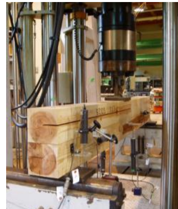
Figure 4. Configurations of built-up beams and actual feature of the bending test.
