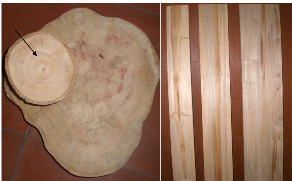
Figure 1. Wood discoloration as a result of secondary heartwood in 5-year-old JUN; compared to 5-year-old conventional teak where the discoloration or secondary heartwood formation was not observed (arrow).
