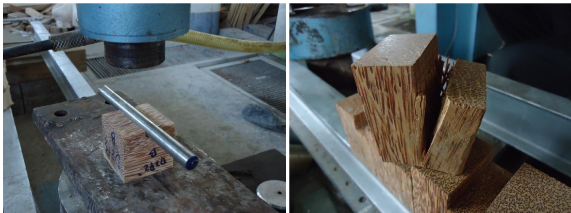
Figure 5. Photos of the test: (a) Dowel bearing test – outer part specimen; and (b) Failure of shear parallel to grain specimen.
