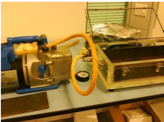
Figure 1. Vacuum-pressure method for impregnation of wood.
