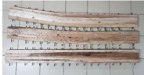
Figure 5. Bolt-laminated specimens after flexural tests
