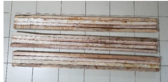
Figure 6. Glue-laminated specimens after flexural tests
