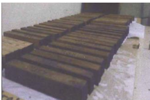
Figure 2. The appearance of teak wood control samples (brighter specimens) and after compregnation treatment (darker specimens) with phenol formaldehyde resin.
