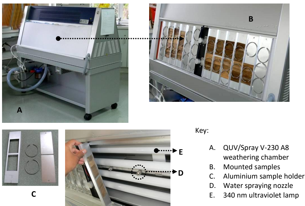
Figure 2. The QUV/Spray V-230 A8 weathering chamber and samples mounted on the aluminium sample holder of the chamber slots.
