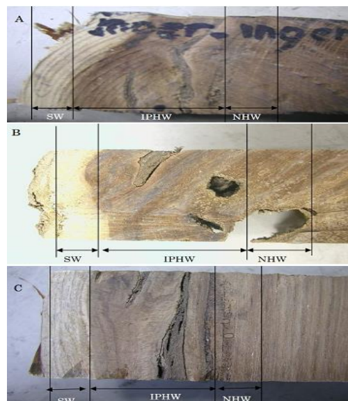
Figure 1. Sampling position on a cross section of heartwood containing included phloem in teak from three trees. Remarks: SW = sapwood, IPHW = included phloem-containing heartwood, NHW = normal heartwood.
