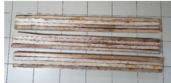
Figure 6. Glue-laminated specimens after flexural tests
