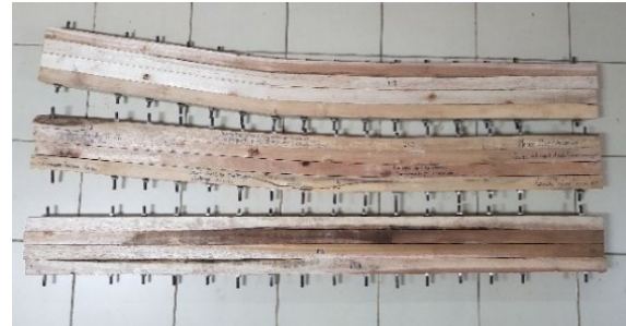
Figure 5. Bolt-laminated specimens after flexural tests
