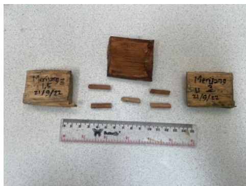
Figure 1. Increment cores and thin wood samples.
