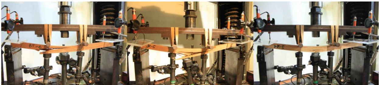
Figure 10. Failure mode of specimen from four point bending test.
