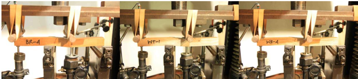
Figure 13. Failure mode of specimen from four points shear test.
