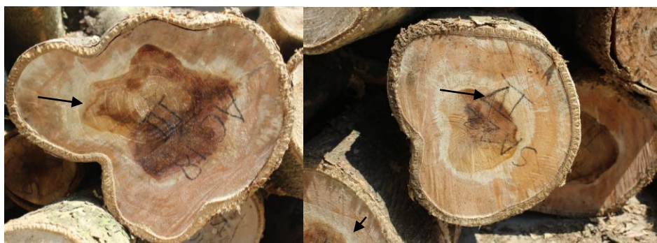
Figure 4. Transition zone (arrows) as it appears in cross sections of all logs cut from 5-year old fast grown teak trees
