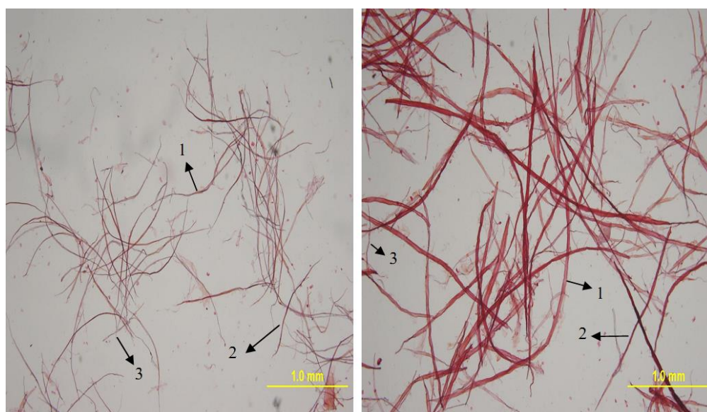
Figure 1. Microscopic images of Acacia nilotica (a) and Pinus merkusii fibers after beating (200~300 CSF). Remark 1 = intact fibers, 2= fiber fragments, 3=fines.
