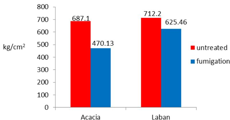
Figure 4. Hardness value of mangium and laban wood.
