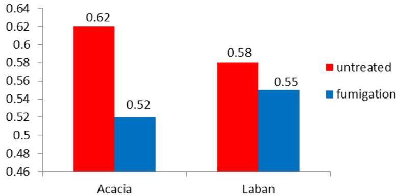
Figure 2. Density of mangium and laban wood.
