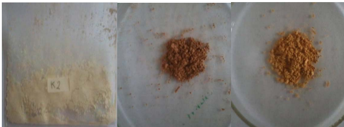
Figure 1. Spray dried-chitosan nanoparticles. Chitosan nanoparticles (A), MBWE-loaded chitosan nanoparticles with 30 min (B) and 60 min (C) of ultrasonication time.
