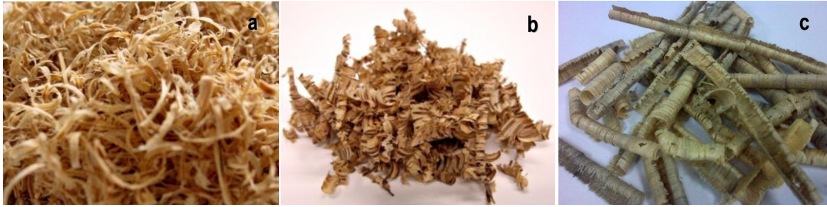
Figure 7. Chip geometry of untreated OPW (a), treated OPW (b), and rubberwood (c).
