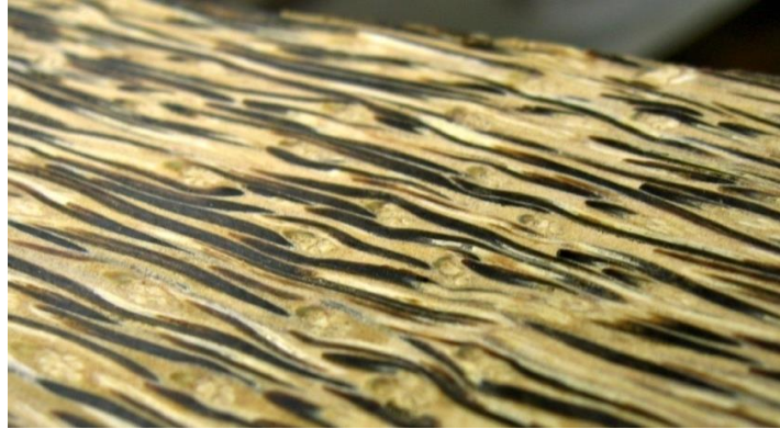
Figure 5. The planed surface of treated OPW showing very smooth surface.
