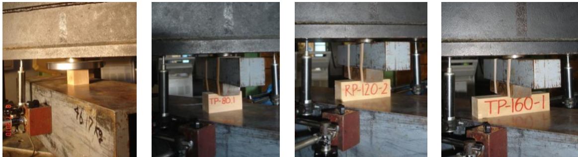
Figure 4. Compression test set-up of tropical timber specimens.
