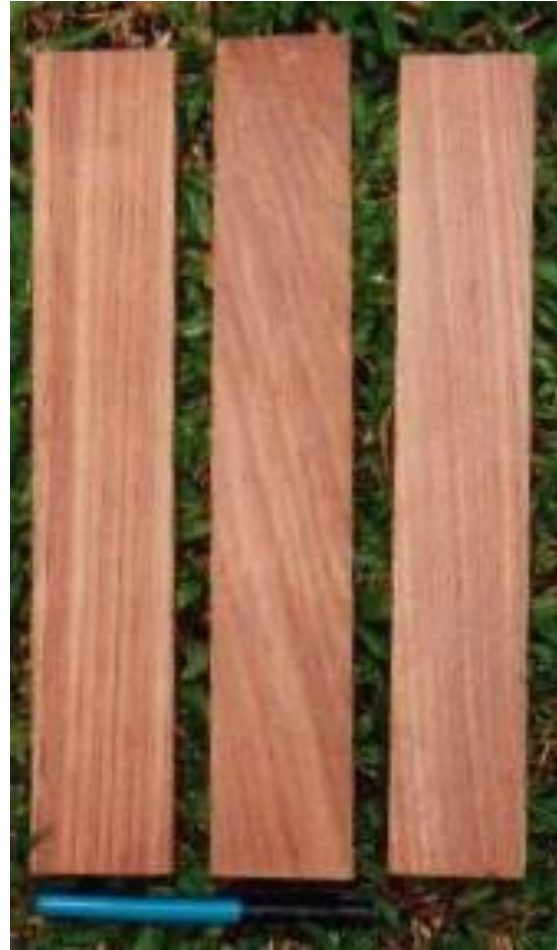
Figure 2. Teak Wood After 5 th Treatment Method.
