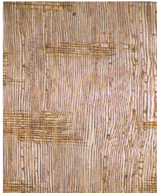
Figure 3. Transverse section of Palele ( Castanopsis javanica ) with solitary and group of vessels, uniseriate rays, and rare of axial parenchyma.
