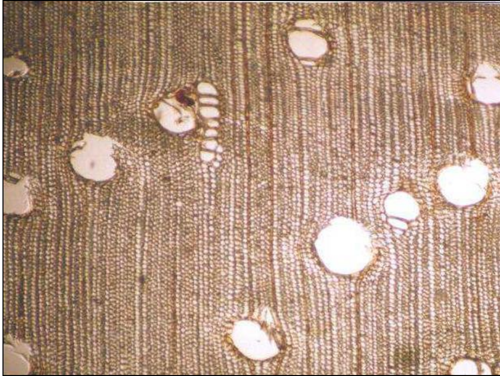
Figure 3. Transverse section of Palele ( Castanopsis javanica ) with solitary and group of vessels, uniseriate rays, and rare of axial parenchyma.
